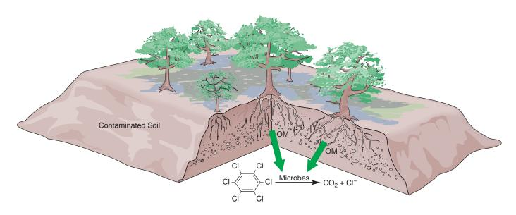
**Figure 41.26** Phytoremediation. A conceptual view of a phytoremediation system, with a cut-away section of the root-soil zone. When organic matter (OM) is released from the plant roots, cometabolic processes can be carried out more efficiently by microbes, leading to enhanced degradation of contaminants. The mineralization of hexachlorobenzene is shown as an example.
