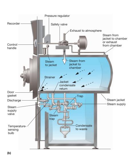
**Figure 7.3** The Autoclave or Steam Sterilizer. (a) A modern, automatically controlled autoclave or sterilizer. (b) Longitudinal cross section of a typical autoclave showing some of its parts and the pathway of steam. From John J. Perkins, *Principles and Methods of Steriliza-tion in Health Science,* 2nd edition, 1969. Courtesy of Charles C. Thomas, Publisher, Springfield, Illinois.
