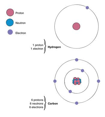
**Figure Al.1** Diagrams of Hydrogen and Carbon Atoms. The electron orbitals are represented as concentric circles.
