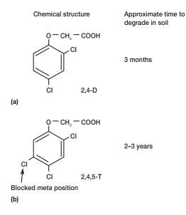
**Figure 41.22** The *Meta* Effect and Biodegradation. Minor structural differences can have major effects on the biodegradability of chemicals. The *meta* effect is an important example. (a) Readily degradable 2,4-dichlorophenoxyacetic acid (2,4-D) with an exposed meta position on the ring degrades in several months; (b) recalcitrant 2,4,5-trichlorophenoxyacetic acid (2,4,5-T) with the blocked meta group, can persist for years.
