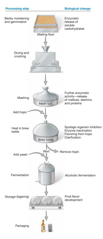
**Figure 40.17 Producing Beer.** To make beer, the complex carbohydrates in the grain must first be transformed into a fermentable substrate. Beer production thus requires the important steps of malting, and the use of hops and boiling for clarification, flavor development, and inactivation of malting enzymes, to produce the wort.
