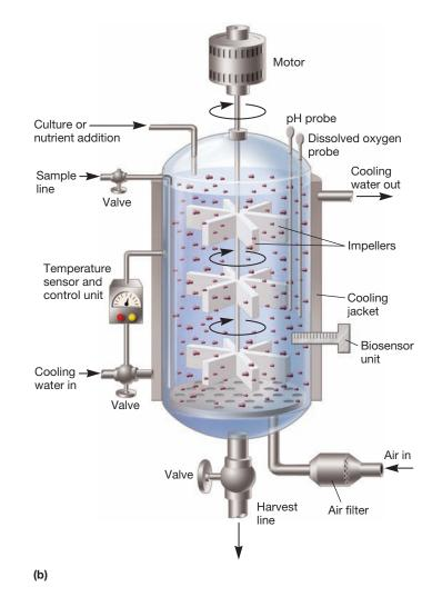
sampling, and process monitoring must be carried out under rigorously controlled conditions. When required, foam control agents must be added, especially with high-protein media. Computers are used to monitor outputs from probes that determine microbial biomass, levels of critical metabolic products, pH, input and exhaust gas composition, and other parameters. Environmental conditions can be changed or held constant over time, depending on the goals for the particular process.
