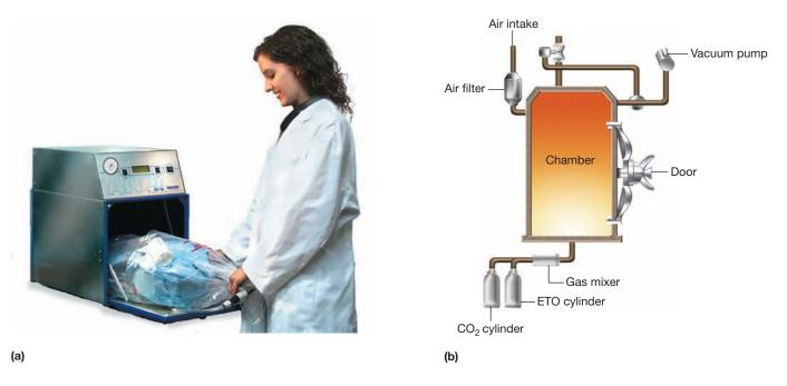
**Figure 7.13** An Ethylene Oxide Sterilizer. (a) An automatic ethylene oxide (EtO) sterilizer. (b) Schematic of an EtO sterilizer. Items to be sterilized are placed in the chamber and EtO and carbon dioxide are introduced. After the sterilization procedure is completed, the EtO and carbon dioxide are pumped out of the chamber and air enters.
