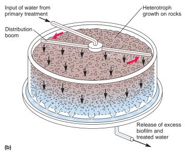
Figure 41.6 Aerobic Secondary Sewage Treatment.
