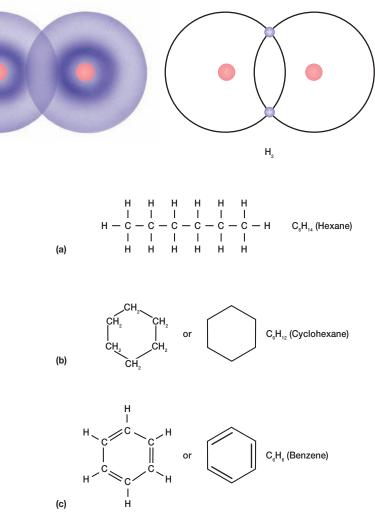
**Figure AI.5** Hydrocarbons. Examples of hydrocarbons that are (a) linear, (b) cyclic, and (c) aromatic.
