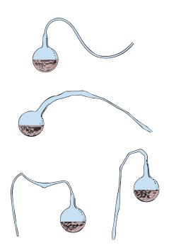
**Figure 1.5** The Spontaneous Generation Experiment. Pasteur's swan neck flasks used in his experiments on the spontaneous generation of microorganisms. *Source: Annales Sciences Naturelle, 4th Series, Vol. 16, pp. 1–98, Pasteur, L., 1861, "Mémoire sur les Corpuscules Organisés Qui Existent Dans L'Atmosphère: Examen de la Doctrine des Générations Spontanées."*
