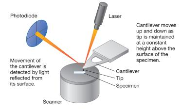
**Figure 2.28** Atomic Force Microscopy—The Basic Elements of an Atomic Force Microscope. The tip used to probe the specimen is attached to a cantilever. As the probe passes over the "hills and valleys" of the specimen's surface, the cantilever is deflected vertically. A laser beam directed at the cantilever is used to monitor these vertical movements. Light reflected from the cantilever is detected by the photodiode and used to generate an image of the specimen.
