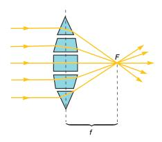
**Figure 2.2** Lens Function. A lens functions somewhat like a collection of prisms. Light rays from a distant source are focused at the focal point *F*. The focal point lies a distance *f*, the focal length, from the lens center.
