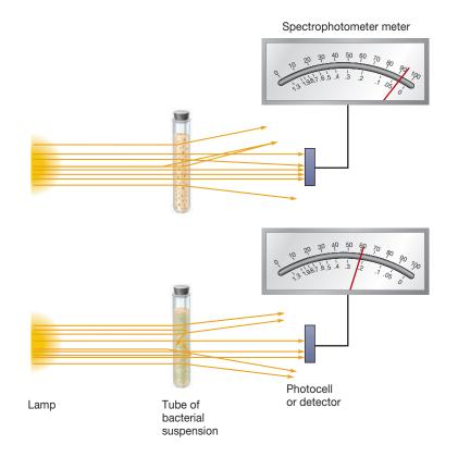
**Figure 6.15** Turbidity and Microbial Mass Measurement. Determination of microbial mass by measurement of light absorption. As the population and turbidity increase, more light is scattered and the absorbance reading given by the spectrophotometer increases. The spectrophotometer meter has two scales. The bottom scale displays absorbance and the top scale, percent transmittance. Absorbance increases as percent transmittance decreases.
