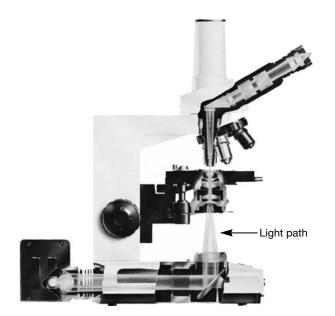
**Figure 2.4** A Microscope's Light Path. The light path in an advanced bright-field microscope (see also figure 2.19).
