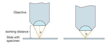
**Figure 2.5** Numerical Aperture in Microscopy. The angular aperture  $\theta$  is 1/2 the angle of the cone of light that enters a lens from a specimen, and the numerical aperture is *n* sin  $\theta$ . In the right-hand illustration the lens has larger angular and numerical apertures; its resolution is greater and its working distance smaller.
