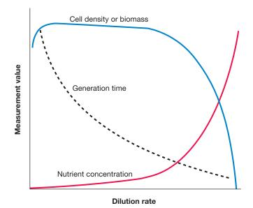
**Figure 6.17** Chemostat Dilution Rate and Microbial **Growth.** The effects of changing the dilution rate in a chemostat.
