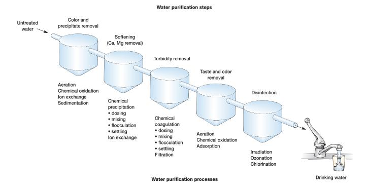
**Figure 41.1** Water Purification. Several alternatives can be used for drinking water treatment depending on the initial water quality. A major concern is disinfection: chlorination can lead to the formation of *d*isinfection-*byp*roducts (DBPs), including potentially carcinogenic *trihalomethanes* (THMs).
