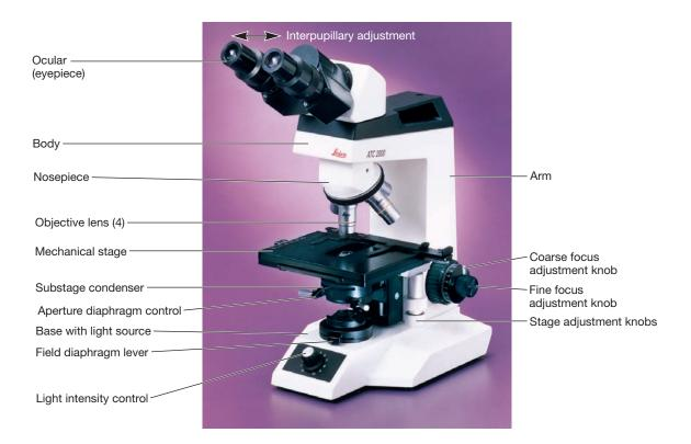
**Figure 2.3** A Bright-Field Microscope. The parts of a modern bright-field microscope. The microscope pictured is somewhat more sophisticated than those found in many student laboratories. For example, it is binocular (has two eyepieces) and has a mechanical stage, an adjustable substage condenser, and a built-in illuminator.
