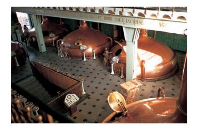
**Figure 40.18** Brew Kettles Used for Preparation of Wort. In large-scale processes, copper brew kettles can be used for wort preparation, as shown here at the Carlsberg Brewery, Copenhagen, Denmark.
