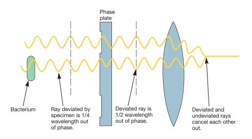
**Figure 2.10** The Production of Contrast in Phase Microscopy. The behavior of deviated and undeviated or undiffracted light rays in the dark-phase-contrast microscope. Because the light rays tend to cancel each other out, the image of the specimen will be dark against a brighter background.
