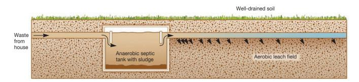
**Figure 41.8** The Conventional Septic Tank Home Treatment System. This system combines an anaerobic waste liquefaction unit (the septic tank) with an aerobic leach field. Biological oxidation of the liquefied waste takes place in the leach field, unless the soil becomes flooded.
