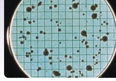
Membrane filters are used in counting microorganisms. This membrane has been used to obtain a total bacterial count using an indicator to color colonies for easy counting.
