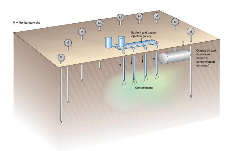
**Figure 41.25** A Subsurface Engineered Bioremediation System. Monitoring and recovery wells are used to monitor the plume and its possible movement. Nutrients and oxygen (as air, peroxide, or other oxygen-releasing compounds) are added to the soil and groundwater to promote more efficient degradation of contaminants.
