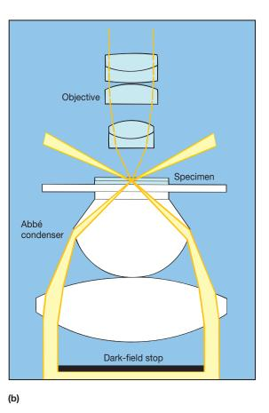
**Figure 2.7** Dark-Field Microscopy. The simplest way to convert a microscope to dark-field microscopy is to place (a) a dark-field stop underneath (b) the condenser lens system. The condenser then produces a hollow cone of light so that the only light entering the objective comes from the specimen.
