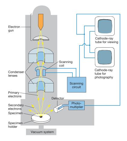
**Figure 2.23** The Scanning Electron Microscope. See text for explanation.
