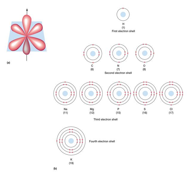
**Figure Al.2** Electron Orbitals. (a) The three dumbbell-shaped orbitals of the second shell. The orbitals lie at right angles to each other. (b) The distribution of electrons in some common elements. Atomic numbers are given in parentheses.
