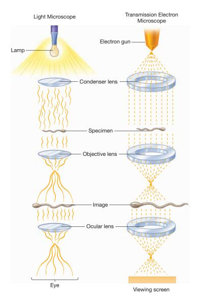
**Figure 2.19** Transmission Electron Microscope Operation. An overview of TEM operation and a comparison of the operation of light and transmission electron microscopes.
