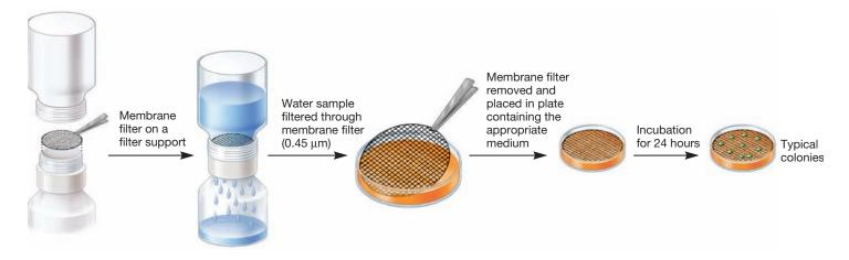
**Figure 6.13** The Membrane Filtration Procedure. Membranes with different pore sizes are used to trap different microorganisms. Incubation times for membranes also vary with the medium and microorganism.
