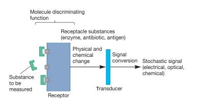
**Figure 41.29 Biosensor Design.** Biosensors are finding increasing applications in medicine, industrial microbiology, and environmental monitoring. In a biosensor a biomolecule or whole microorganism carries out a biological reaction, and the reaction products are used to produce an electrical signal.
