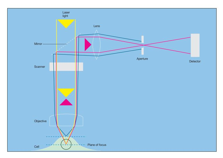
**Figure 2.26** A Ray Diagram of a Confocal Laser Scanning Microscope. The yellow lines represent laser light used for illumination. Red lines symbolize the light arising from the plane of focus, and the blue lines stand for light from parts of the specimen above and below the focal plane. See text for explanation.
