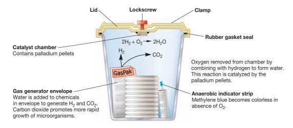
**Figure 6.24** The GasPak Anaerobic System. Hydrogen and carbon dioxide are generated by a GasPak envelope. The palladium catalyst in the chamber lid catalyzes the formation of water from hydrogen and oxygen, thereby removing oxygen from the sealed chamber.
