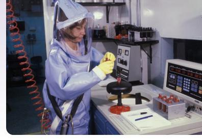
This laboratory worker at the Centers for Disease Control and Prevention (CDC) is in the highest level of isolation (Level 4) to avoid contact with microorganisms and to prevent their escape into the environment.
